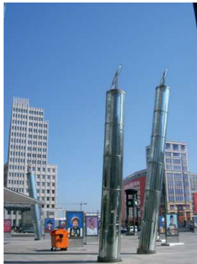
Light Pipes, Berlin Potsdamer Platz Three imposing columns of light extend upwards from Potsdamer Platz. These "Light Pipes" transport sunlight into the regional train station below, illuminating selected areas with natural daylight. At night, the pipes are artificially illuminated from inside. Building owner Deutsche Bundesbahn.
