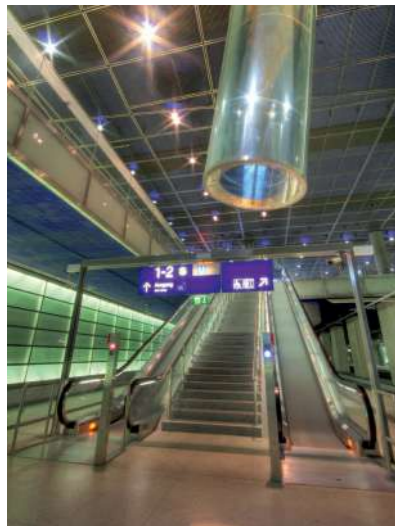
Light Pipes, Berlin Potsdamer Platz Three imposing columns of light extend upwards from Potsdamer Platz. These "Light Pipes" transport sunlight into the regional train station below, illuminating selected areas with natural daylight. At night, the pipes are artificially illuminated from inside. Building owner Deutsche Bundesbahn.
