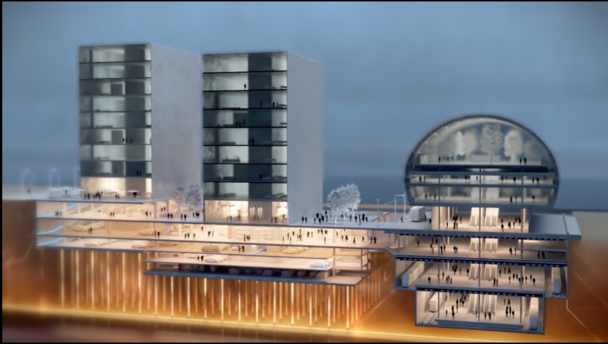
A thick common ground servicing several buildings at once.
